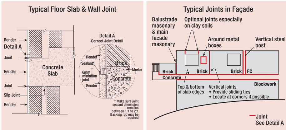
Left: Floor slab and wall joint systems are fundamental to crack-free buildings.
