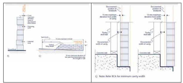
Based on AS 3700 - Masonry structures - Table 11.1 Tolerances in masonry construction
