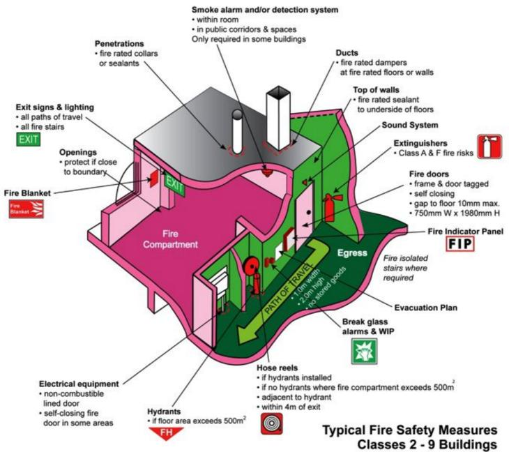
Basic BCA rules for buildings less than 25m high Sprinklers & emergency warning systems required if height exceeds 25m
